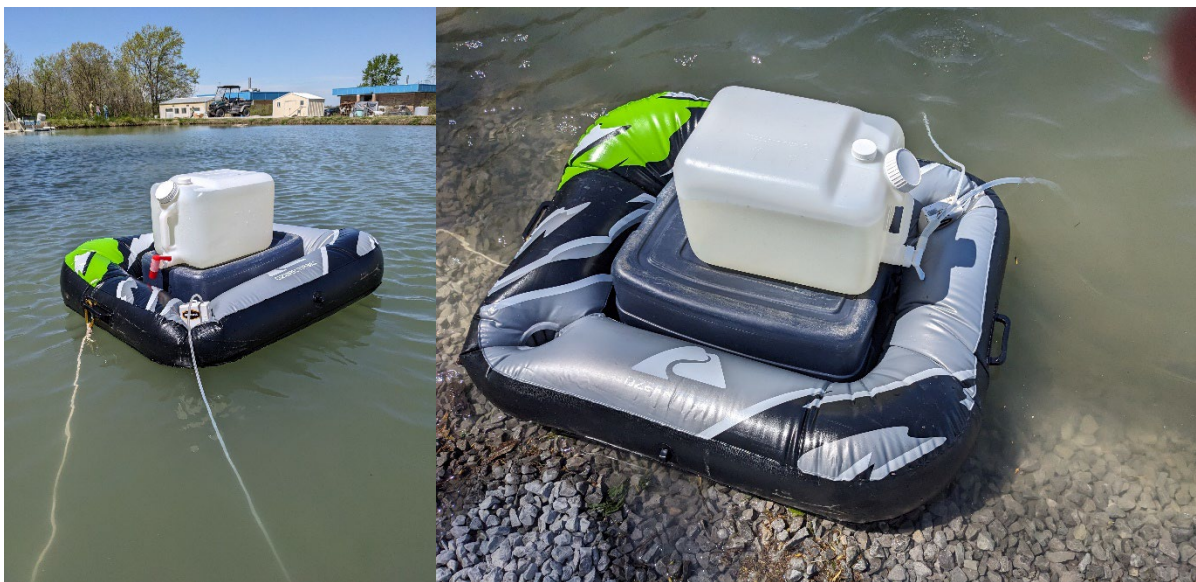
Fig. 3. Square raft (solid bottom) with Rubbermaid container platform.
