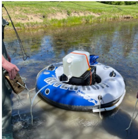
Fig. 1. Inflatable tube with mesh bottom (design selected for use).
