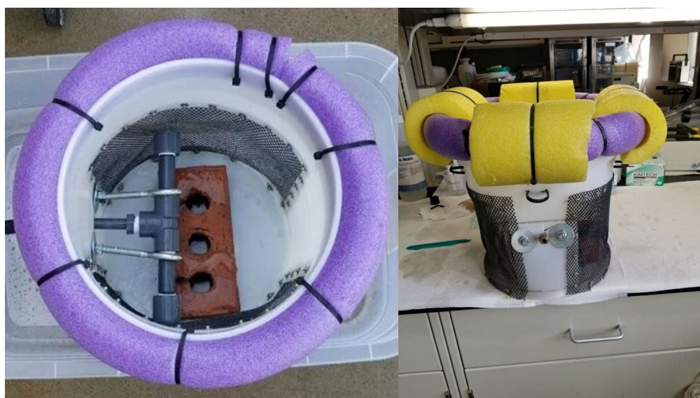
Fig. 2 Standard pool noodle and large clamp noodles secured to bucket boom.
