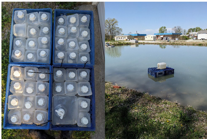
Fig. 2. Milk crates and various sizes of carboys (inflated with air).
