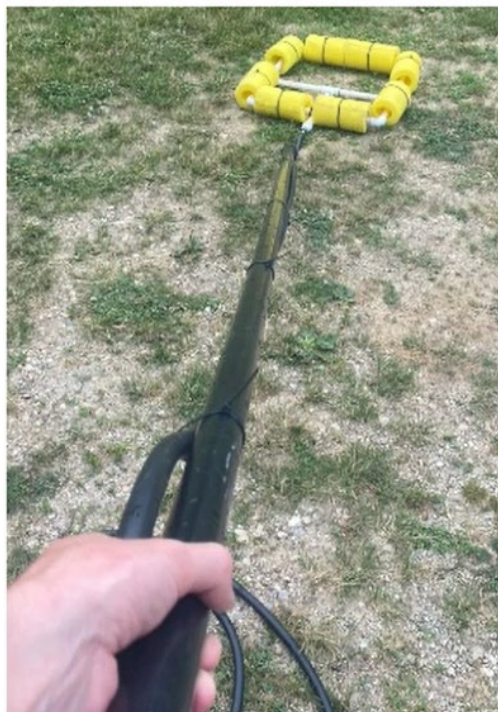
Fig. 3 PVC wand made of spray gun, PVC pipe and fitting, and platform boom.
