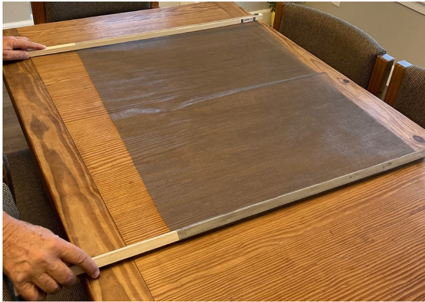
A simple kick net made by stapling window screen to scrap wood.
